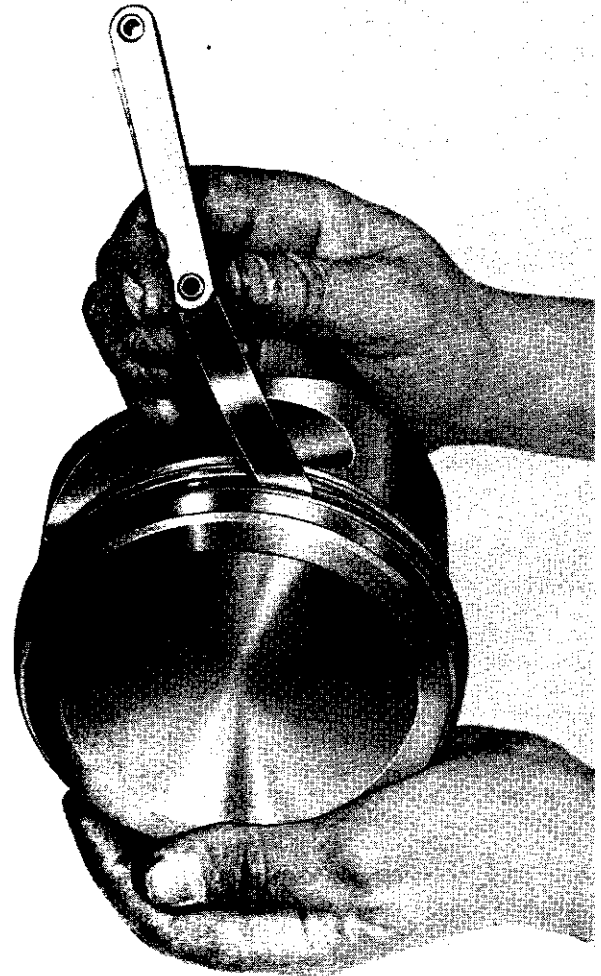
Figure 36. Inspecting Ring Side Clearance
