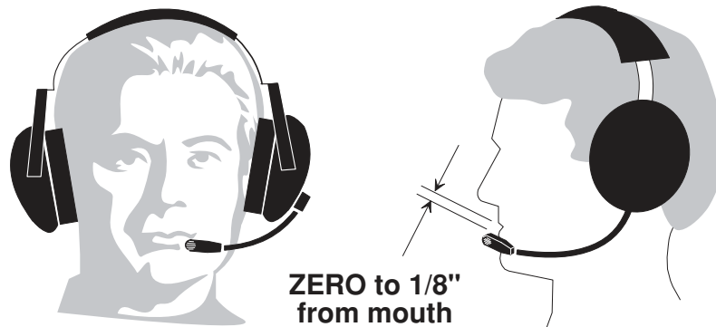
Figure 14 - Correct Positioning of Boom and Microphone
